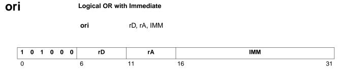
The contents of register rA are ORed with the extended IMM field, sign-extended to 32 bits; the result is placed into register rD.
